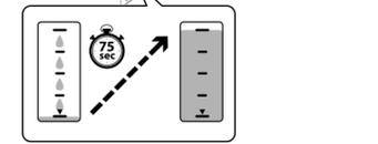
When you insert the ink bottle into the filling port for the correct color, ink starts pouring and the flow stops automatically when the ink reaches the upper line.
